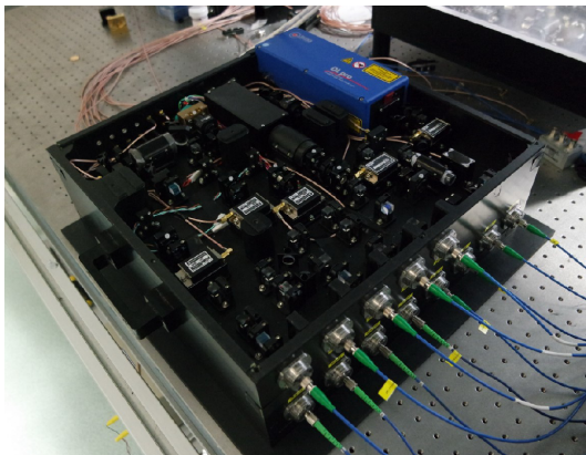
Figure 1: Photograph of the laser system. To improve the degree of integration, a series of the miniaturized optical components were designed.
